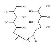
n is 4 or 6 and R is represented by C<sub>12</sub>, C<sub>14</sub>, C<sub>16</sub>, and C<sub>18</sub>
